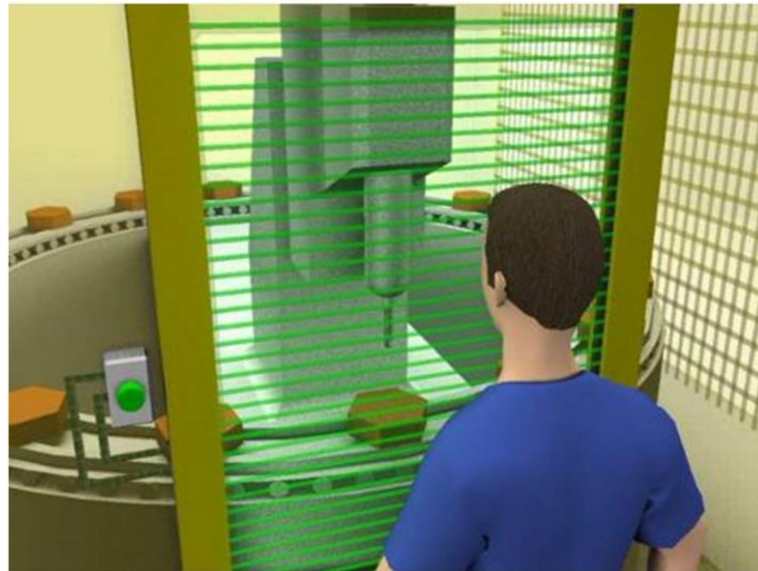
Fig 5 - Operating point protection on drilling machines
